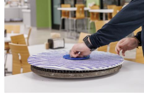
3. Attach the paired pads onto the autoscrubber pad driver and secure according to the autoscrubber manufacturer's instructions.
