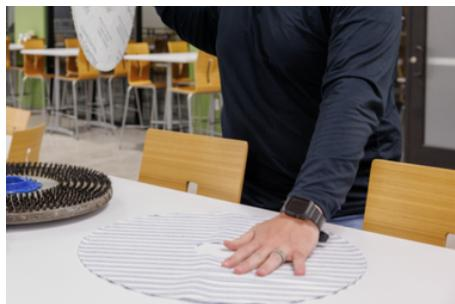
1. Place the autoscrubber pad cleaning side down onto a flat surface.
