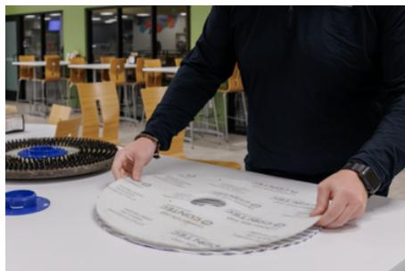
2. Attach the appropriate Connector pad to the back of the autoscrubber pad.
